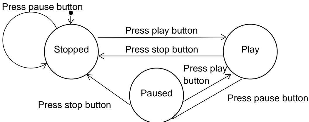
The event (press pause when state is Stopped) that does not cause any change in state is indicated by the circular arrow.
